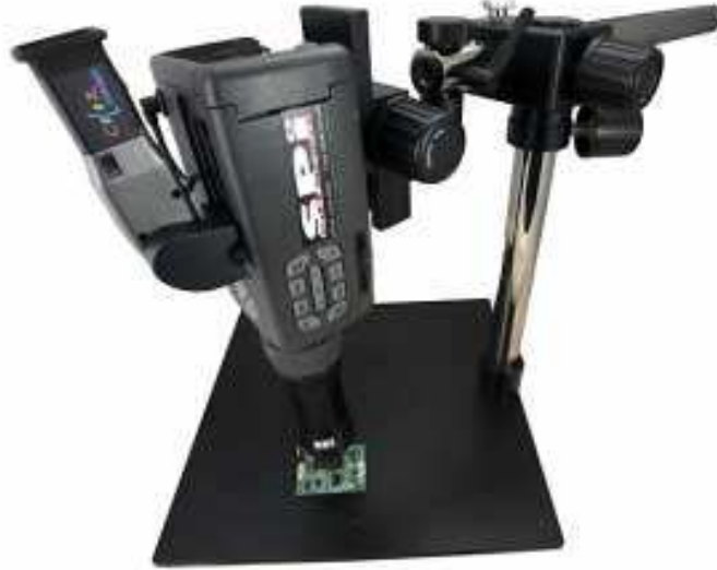
Figure 3.6 Infrared (IR) thermal microscopy setup.
